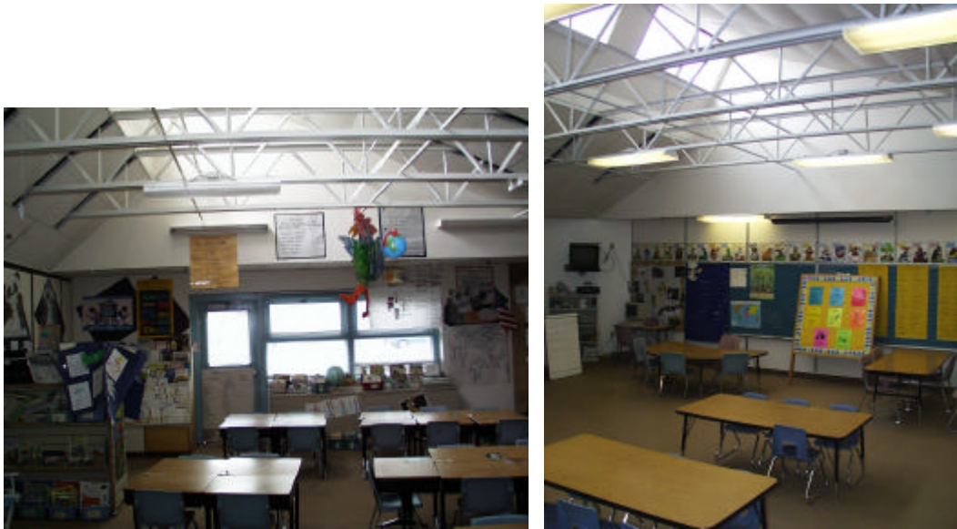
Figure 8: Interior of Fort Collins school with South Facing Monitor Skylight
